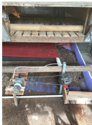
Fig. 11. Motor DC testing
