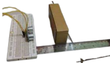
Fig. 10. Ultrasonic sensor testing of ruler
