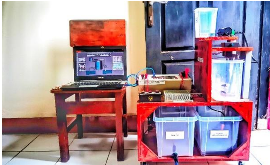
Fig. 5 Fabricated PLC-based water-treatment automation prototype
