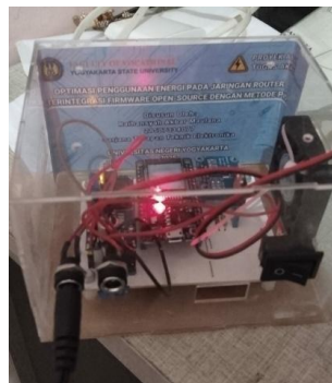
Fig. 5 Power optimization controller built with ESP32 and INA219, enclosed for protection.
