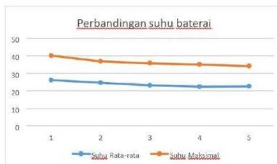
**Fig. 7.** Perbandingan suhu battery jika suhu AC 25°C
