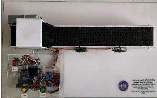
Gambar 5. Training Kit Konveyor berbasis Arduino Uno
