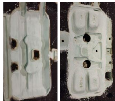
Figure 12. Coating of the second layer in the O3
