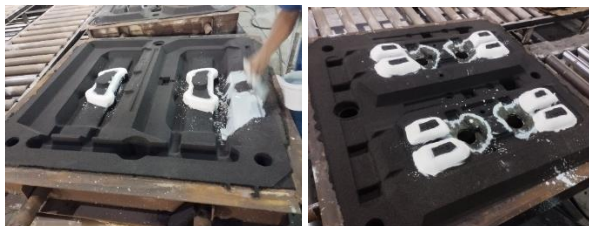
Figure 5. First layer coating of group O1
