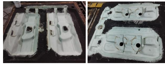
Figure 5. Second layer coating of group O1
