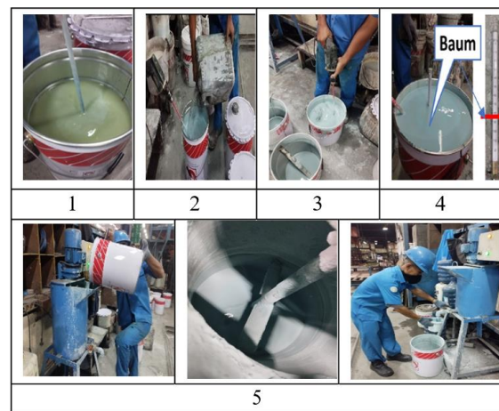
Figure 21. Coating preparation after using CPM
