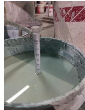
Figure 19. Coating settling after 10 minutes
