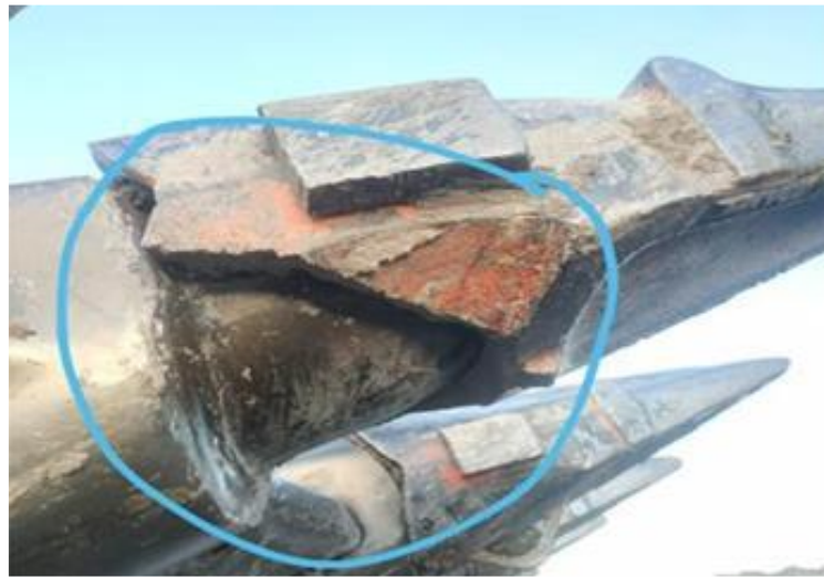
Figure 1. The tooth bucket bottom was broken
