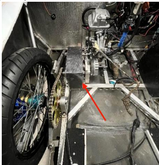
Figure 5. Installation of transmission on the chassis
