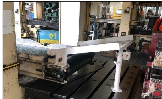
Figure 7. Extension Conveyor Fitting Process
