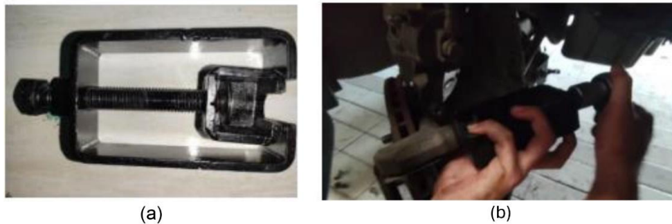
Figure 6. Caliper sliding tool: (a) prototype and (b) functional test
