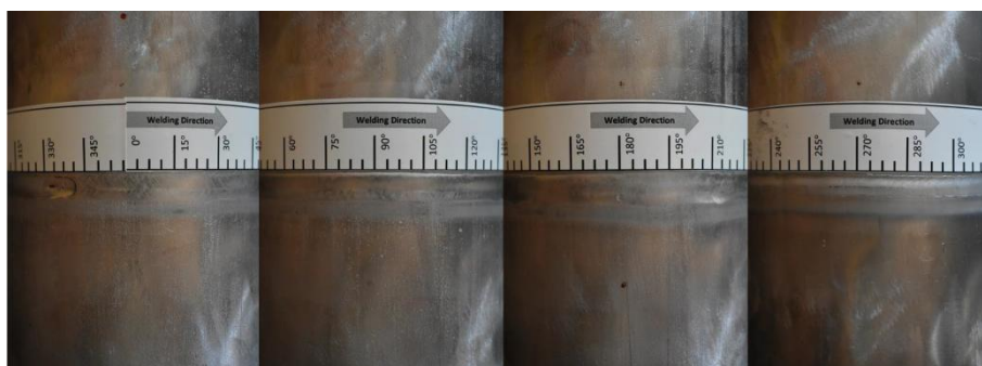
Figure 8. The results of the weld using the orbital pipe welding prototype
