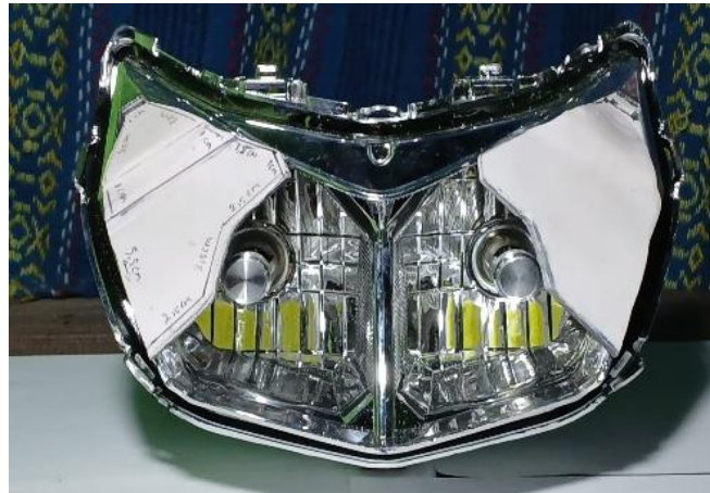
Figure 2. Implementation of the acrylic shield/baffle inside the reflector assembly
