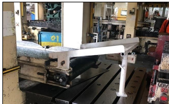
Figure 7. Extension Conveyor Fitting Process
