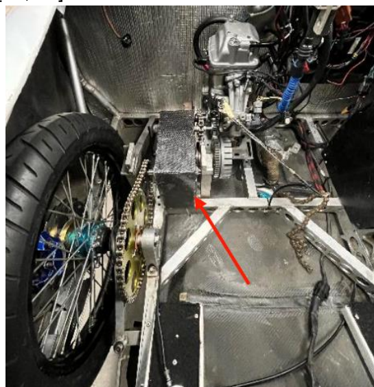
Figure 5. Installation of transmission on the chassis
