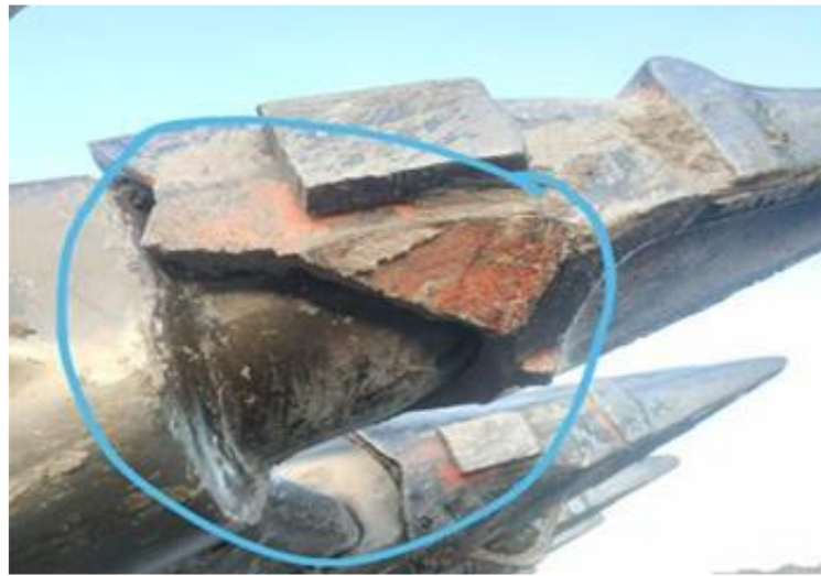
Figure 1. The tooth bucket bottom was broken
