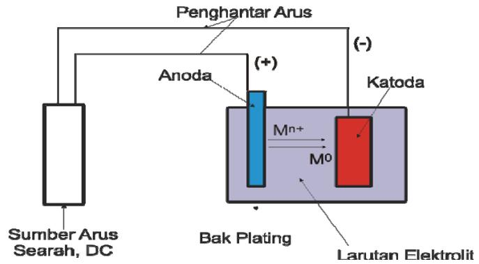
Gambar 1. Skema Proses *Electroplating*
