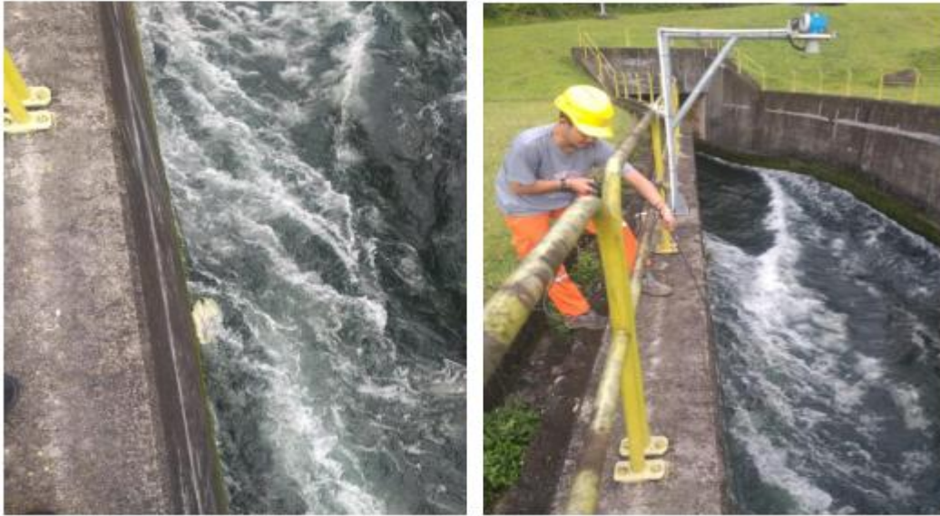
Figure 1. The process of measuring the depth of the Outflow at Singkarak Hydroelectric Power Plant
