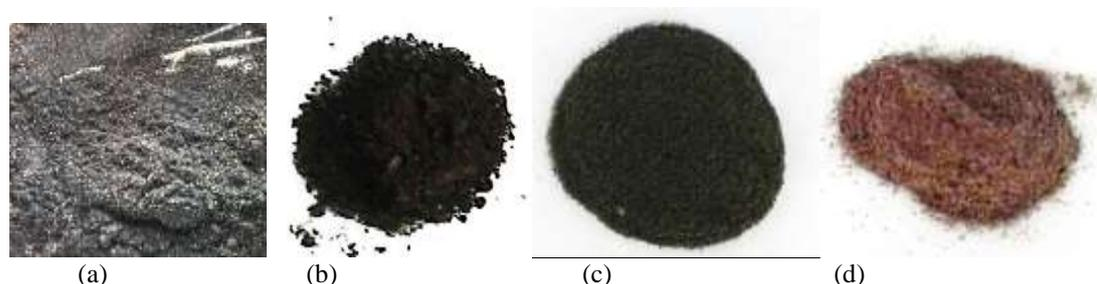
Figure 2. (a) iron sand, (b) M (magnetite resulted from magnetic separation before coating), (c) MSA (magnetic after silica coating calcined in  $80^{\circ}\text{C}$ ), and (d) MSB (magnetic after silica coating calcined in  $350^{\circ}\text{C}$ )
