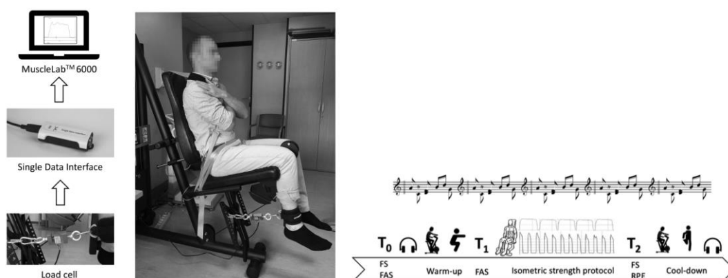
Figure 4. Illustration of a force measurement device and a series of test sessions that include the Feeling Scale (FS), Felt Arousal Scale (FAS), and Rate of Perceived Exertion (RPE) (Source: Greco et al., 2022)
