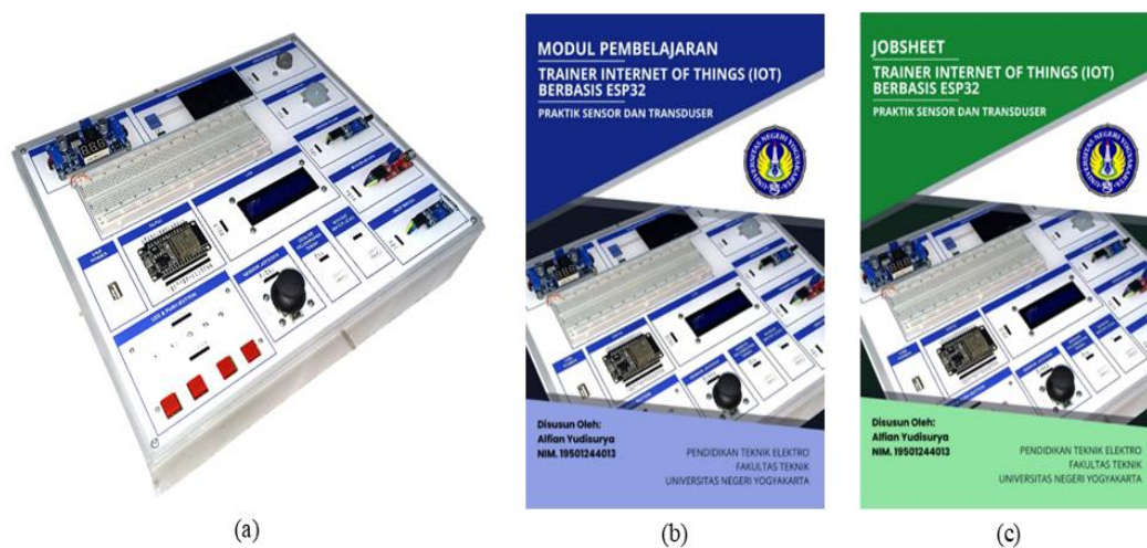
Figure 2. Final IoT Trainer Product: (a) Trainer Unit, (b) Learning Module, (c) Jobsheets
