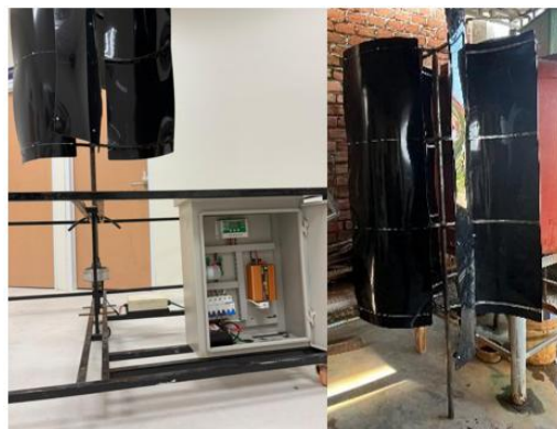
Figure 2. Laboratory-scale Savonius wind turbine prototype showing (a) assembled system with frame and electrical panel, and (b) detailed view of the Savonius rotor structure.
