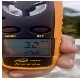
Figure 3. Wind speed measurement using a digital anemometer installed at rotor height.
