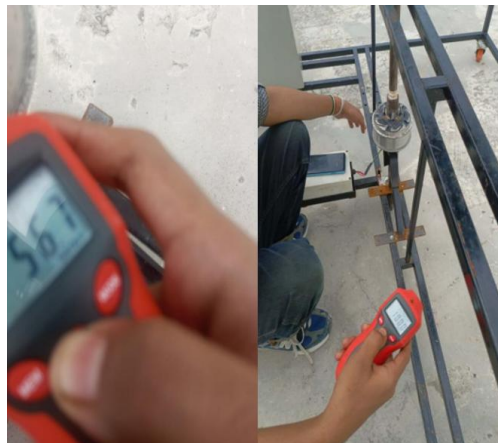
Figure 4. Measurement of rotor rotational speed using a non-contact digital tachometer.
