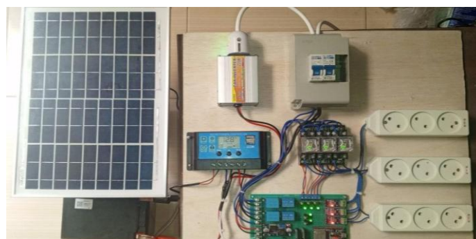
Figure 4. Automatic transfer switch (ATS) prototype design
