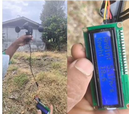
Figure 6. Measuring wind speed using an anemometer
