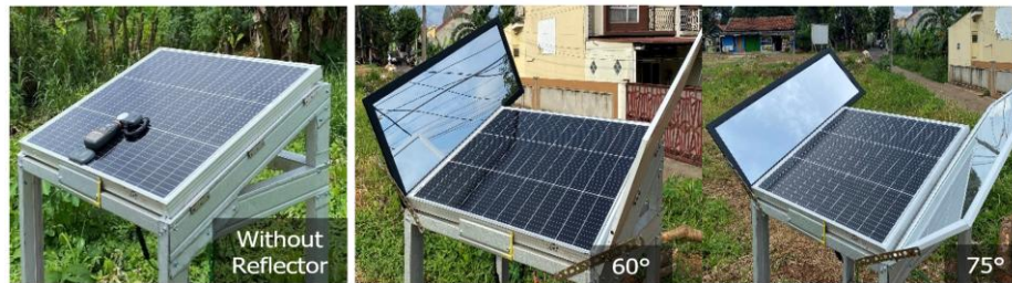
Figure 3. Monocrystalline solar panel without reflector and at tilt angles of 60° and 75°
