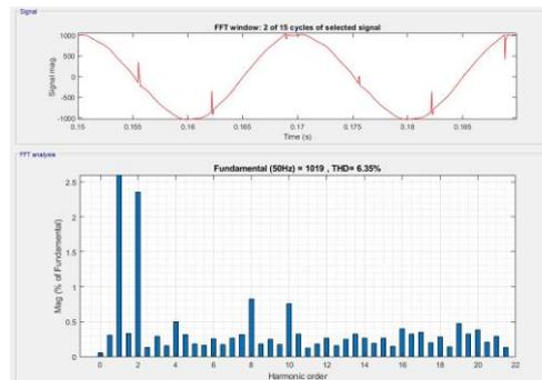
**Fig. 10.** FFT Analysis result after filter installation on 600KW DC motor load
