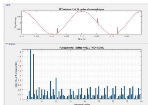
**Fig. 9.** FFT Analysis result after filter installation on 450KW DC motor load
