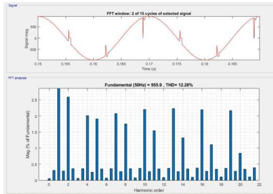
**Fig. 7.** FFT analysis results on DC motor 600KW load
