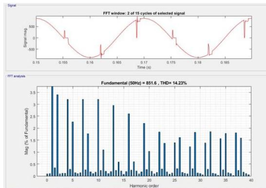
Fig. 6. FFT analysis results on DC motor 450KW load
