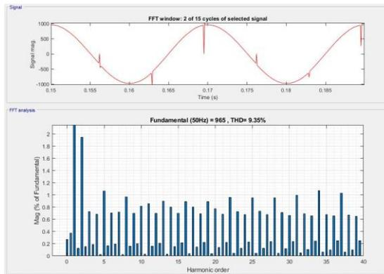
Fig. 5. FFT analysis results on DC motor 400KW load
