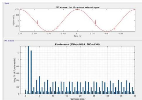
**Fig. 8.** FFT analysis result after filter installation on 400KW DC motor load
