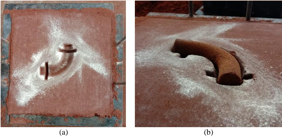
Fig. 5. (a) Sand molding; (b) The sand core fall into sand cavity
