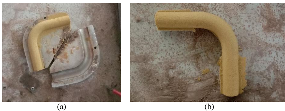
Fig. 9. (a) Core box revision and (b) Revised sand core
