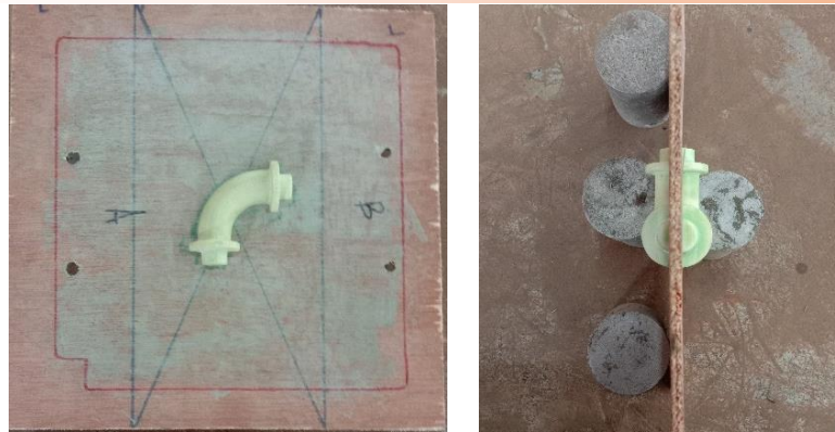
Fig. 3. Assembled patterns in wood plate
