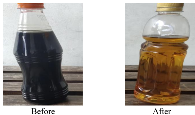
Fig. 8. Photograph of Isopropanol before and after the impinging scrubber
