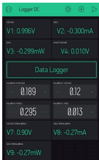
Fig. 3. Example of measurement readout inside the Blynk system interface
