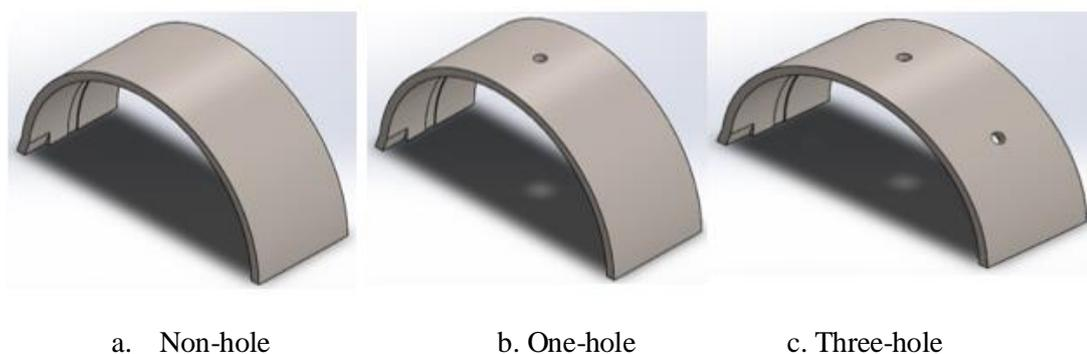
Fig. 2. Various thrust-bearing designs
