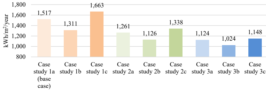
Figure 5. Average Solar Radiation Simulation Results / Year on West - East Site Orientation.
