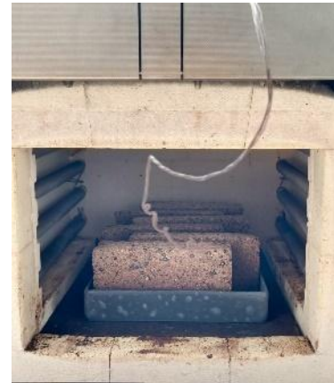
Figure 5. After Firing Process of Samples Using a Chamber Furnace
