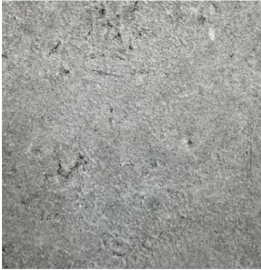
Figure 6. The visual appearance of the surface of the unburned sample appears gray, similar to the color of cement
