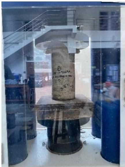
Figure 1. Compressive strength test on concrete
