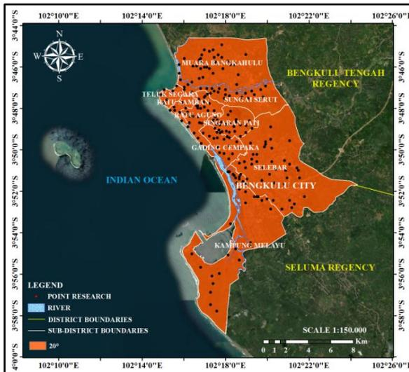
Figure 22. Distribution Map of Inner Friction Angle ( $\phi$ ) Values in Clay Soil Layer
