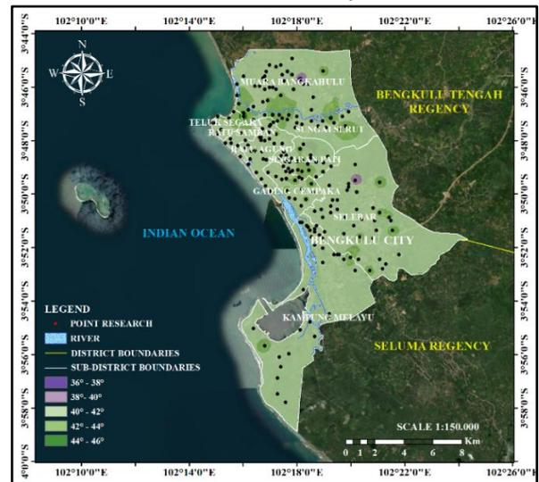
Figure 25. Distribution Map of Inner Friction Angle ( $\phi$ ) Values in Hard Rock Layer
