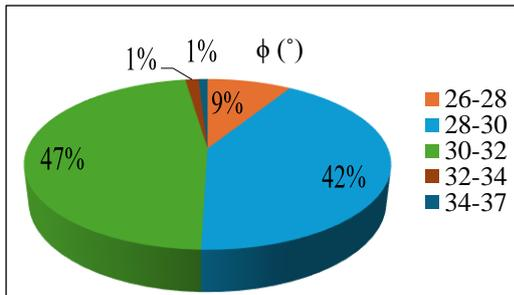
Figure 9. Percentage Diagram of Inner Friction Angle (φ) Data on Sand Layer
