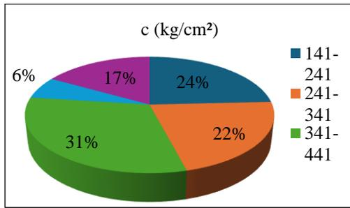
Figure 8. Percentage Chart of Cohesion Data (c) on Clay Soil
