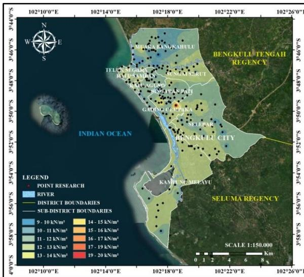
Figure 20. Distribution Map of Cohesion Value (c) in Clay Soil Layer
