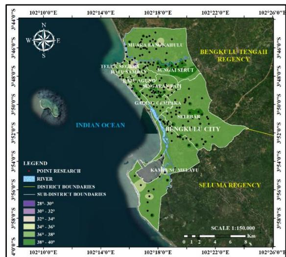
Figure 24. Distribution Map of Inner Friction Angle ( $\phi$ ) Values in Medium Rock Layer
