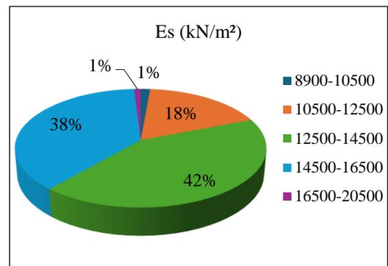
**Figure 6.** Data Percentage Diagram of Modulus of Elasticity (Es) in medium rock layers
