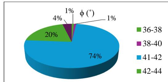
Figure 13. Diagram of Percentage Data of Inner Friction Angle (φ) in Hard Rock Layer
