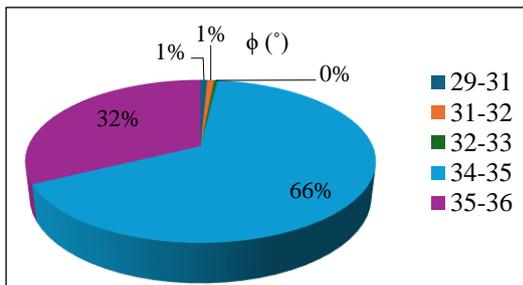
Figure 11. Diagram of Percentage Data of Inner Friction Angle (φ) in Soft Rock Layer
