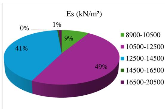
**Figure 3.** Percentage Chart of Modulus of Elasticity (Es) Data on Sand Layer
