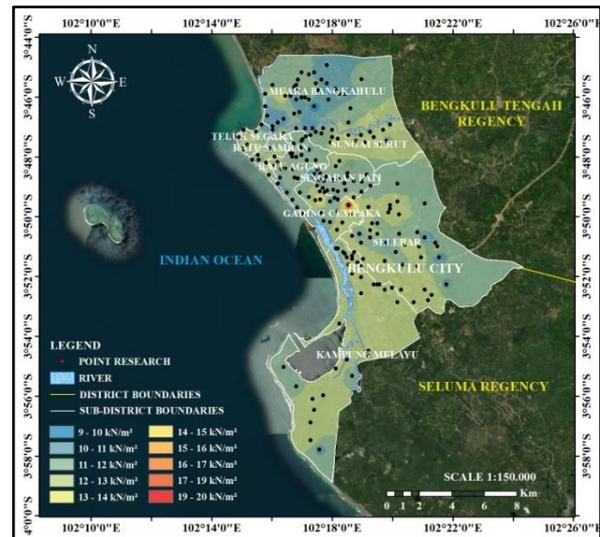
Figure 21. Distribution Map of Inner Friction Angle (φ) Values in Sand Soil Layer
