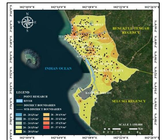
Figure 19. Distribution Map of Modulus of Elasticity ( $E_s$ ) Values in Hard Rock Layers
