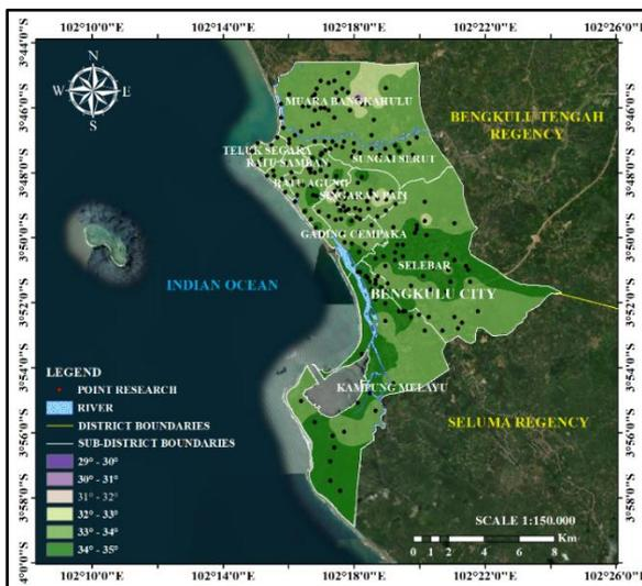
Figure 23. Distribution Map of Inner Friction Angle ( $\phi$ ) Values in Soft Rock Layer
