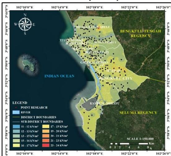
Figure 17. Distribution Map of Modulus of Elasticity ( $E_s$ ) Values in Soft Rock Layers
