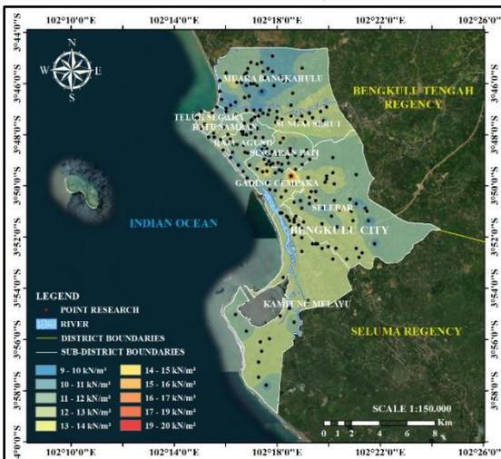
Figure 16. Distribution Map of Modulus of Elasticity ( $E_s$ ) Values in Clay Soil Layer
