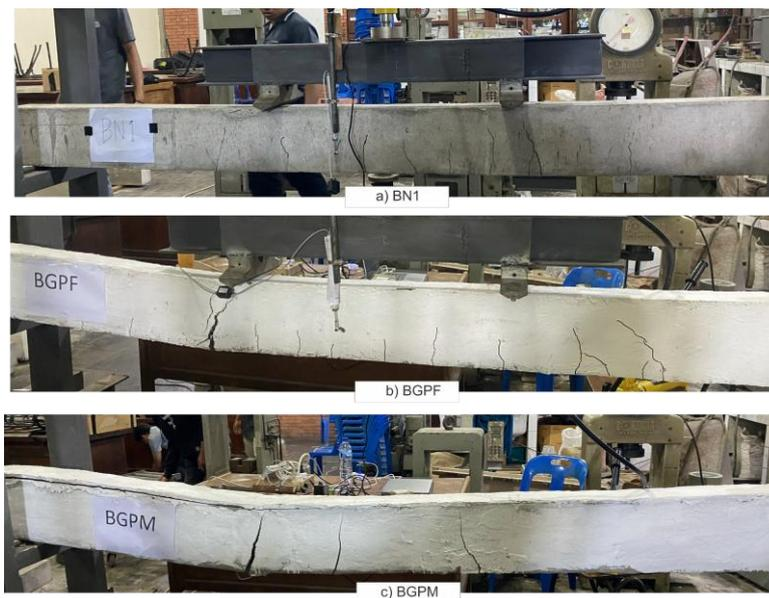
**Figure 5.** Flexural geopolymer concrete beam test result of a) normal concrete (BN), b) Fly ash (BGPF) & c) Metakaolin (BGPM)
