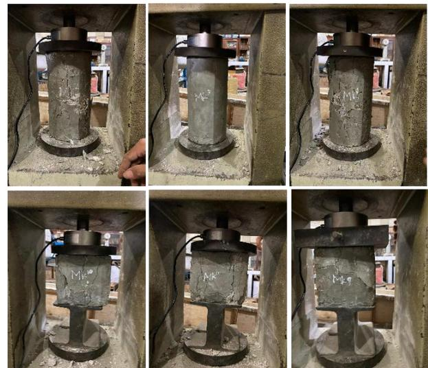
**Figure 4.** Test results of Metakaolin geopolymer concrete cylinders and cubes
