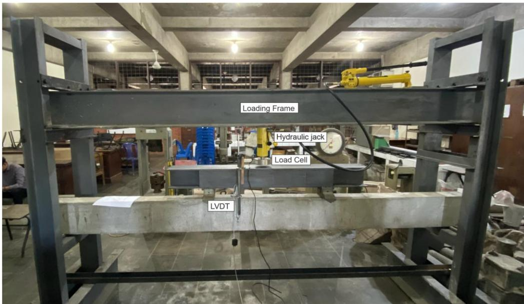
**Figure 2.** Setup flexural test in Laboratory
