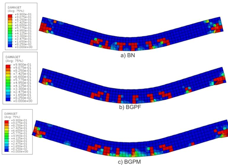
**Figure 6.** Flexural geopolymer concrete beam FEM Analysis of a) normal concrete (BN), b) Fly ash (BGPF) & c) Metakaolin (BGPM)
