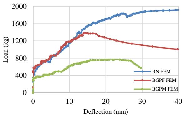
Figure 8. FEM analysis load and deflection graph
