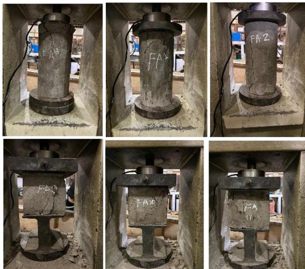
**Figure 3.** Test results of Fly Ash geopolymer concrete cylinders and cubes
