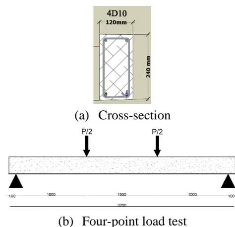
**Figure 1.** Loading flexural beam test method units in mm
