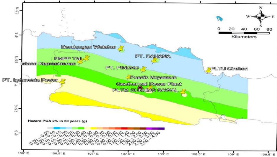
Figure 4. Earthquake Hazard Map due to Megathrust
