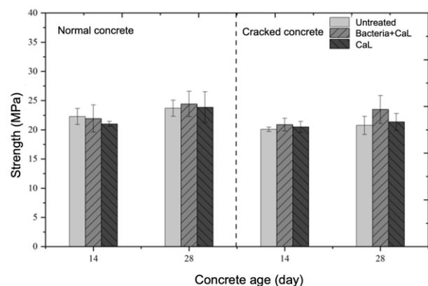
**Figure 6.** Compressive strength test results for variations of concrete samples aged 14 and 28 days
