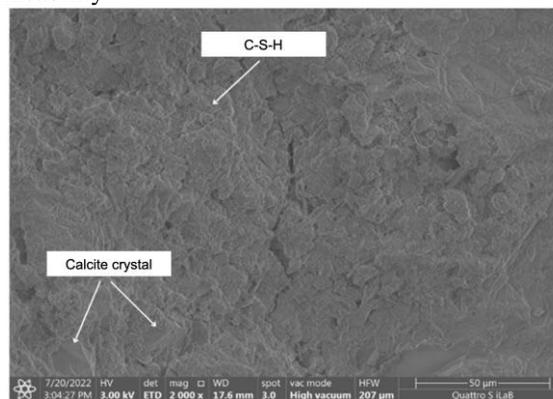
Figure 9. SEM test results on bacteria+CaL concrete with a magnification of 2,000 times
