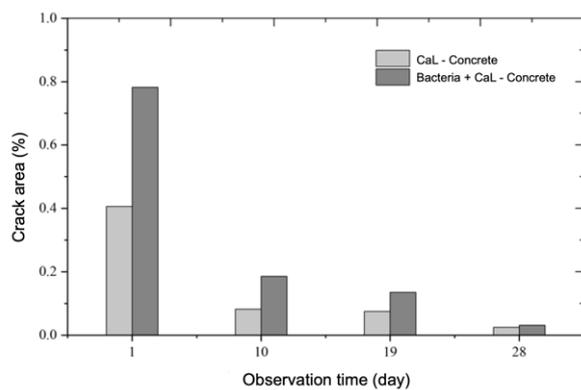
Figure 5. Graph of crack area per total area at each concrete age
