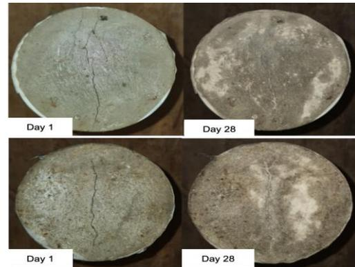
Figure 3. Photo of normal bacteria+CaL concrete (top) and photo of normal CaL concrete (bottom)
