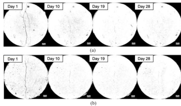
Figure 4. ImageJ processing results on normal bacteria+CaL concrete (a) and normal CaL concrete (b)
