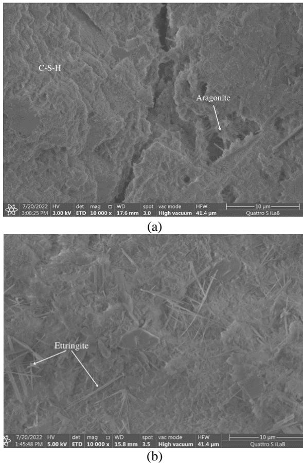
**Figure 10.** SEM testing on bacterial+CaL concrete (a) and normal concrete (b)
