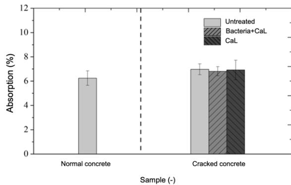
Figure 8. Concrete absorption capacity test results
