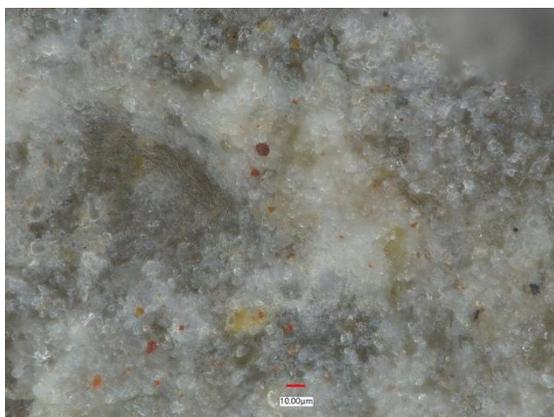
**Figure 11.** Observation results on the concrete surface with 1000 times magnification using VHX-7000
