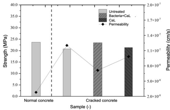
Figure 7. The relationship between compressive strength and concrete permeability
