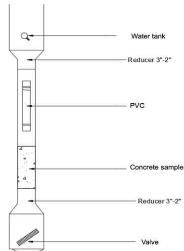
Figure 1. Concrete permeability testing scheme
