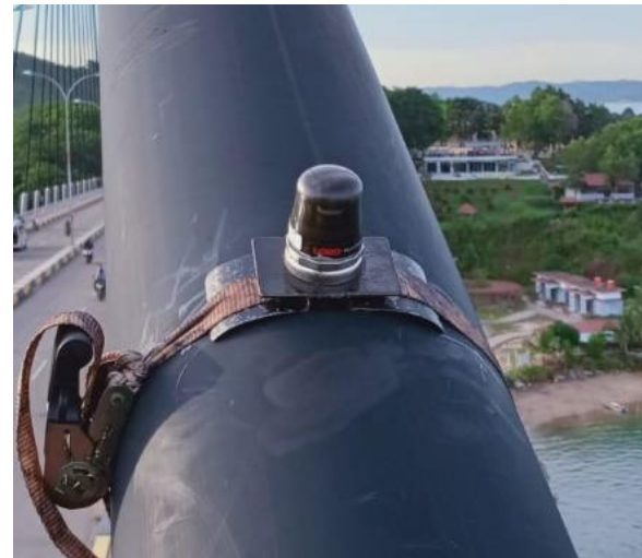
Figure 4. The accelerometer is attached to the cable.
