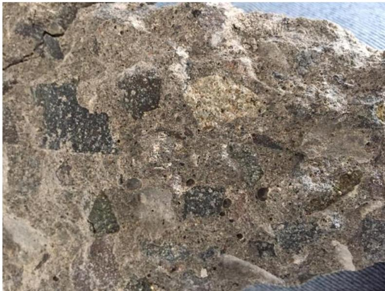
**Figure 10.** Air cavity pattern in concrete
