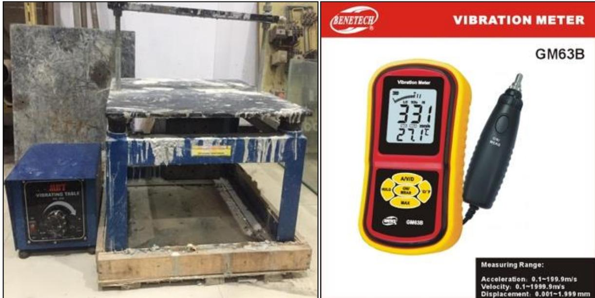
Figure 3. (a) MBT vibrating table CO-410; (b) Vibration Meter GM63B
