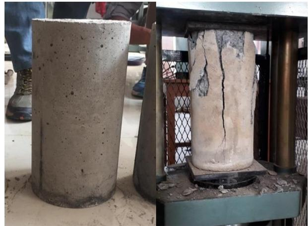
**Figure 9.** (a) Concrete air void (b) After compressive strength test
