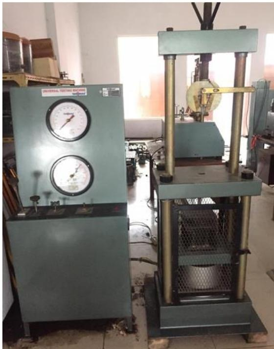
Figure 4. Universal Testing Machine type TC-32
