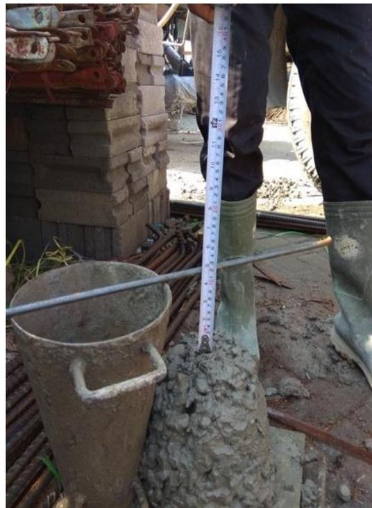
Figure 5. Slump Test
