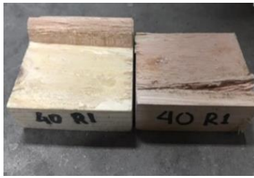
Figure 15. Damage to wood adhesion test.
