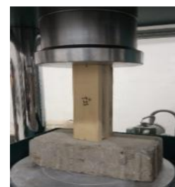
Figure 9. Scheme of compressive strength test.
