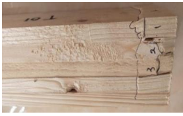
Figure 17. Compression and shear cracking damage.
