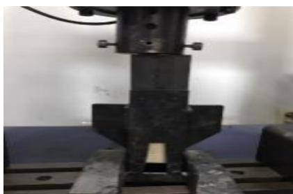
Figure 8. Scheme of adhesive strength test.
