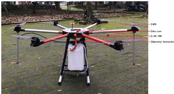
Figure 11. drone design results
