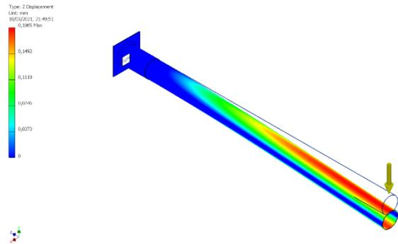
Figure 9. Displacement total
