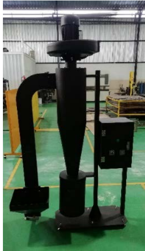
Gambar 18. Purwarupa Mesin Destoner Kopi
