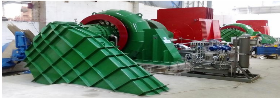
Figure 1. Horizontal Francis Turbine with a Capacity of 6 MW
