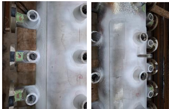
Figure 4. Liquid penetrating testing results of the repaired sparger header
