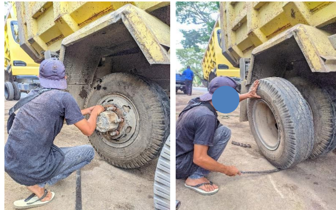
Figure 1. Unnatural Working Posture When Installing Truck Tires
