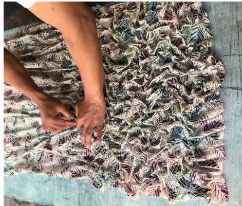
Figure 11. Fabric Smocking Process
