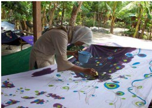
**Gambar 3. Teknik memoleskan larutan cat remazol**
