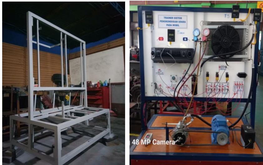
Figure 3. Ready-to-install simulator support frame and simulator
