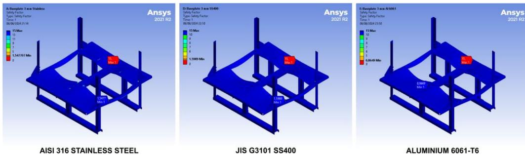
Fig. 16. Safety factor simulation results of 3 mm-thick plate
