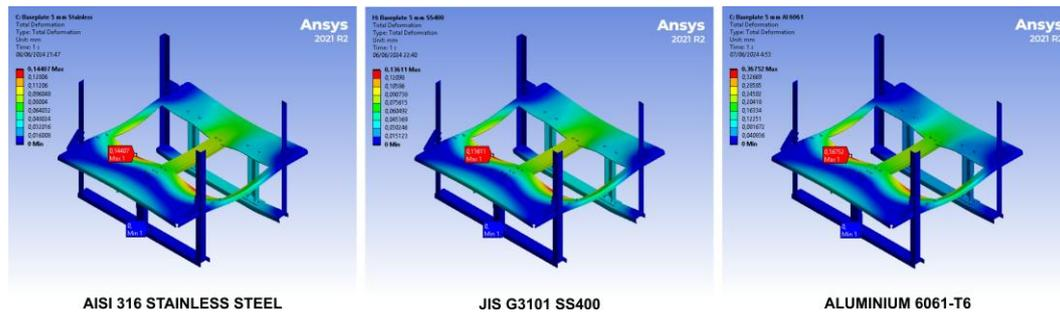
Fig. 14. Deformation simulation results of 5 mm-thick plate
