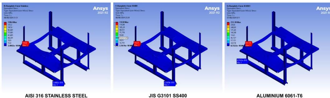
**Fig. 9** Von Mises stress simulation results 4 mm-thick plate
