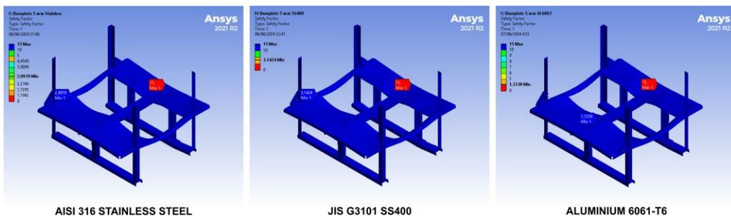
Fig. 18. Safety factor simulation results of 5 mm-thick plate
