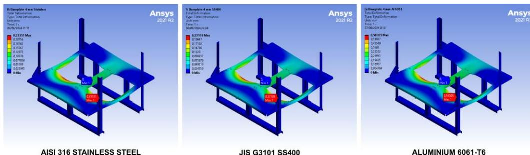
**Fig. 13.** Deformation simulation results of 4 mm-thick plate
