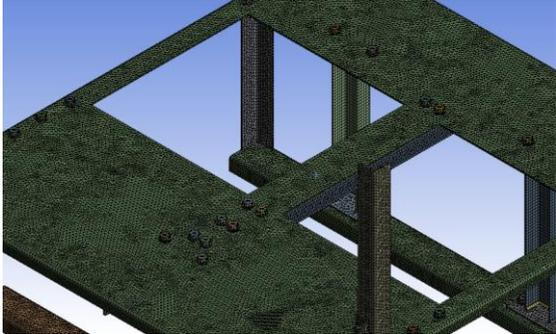
Fig. 3. Process meshing on baseplate model
