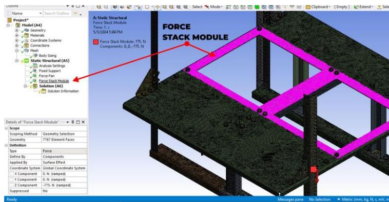
Fig. 6. Force settings for stack module load
