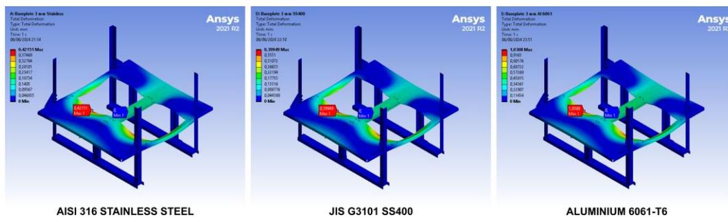
**Fig. 12.** Deformation simulation results of 3 mm-thick plate
