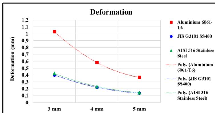
Fig. 15. Maximum deformation simulation result
