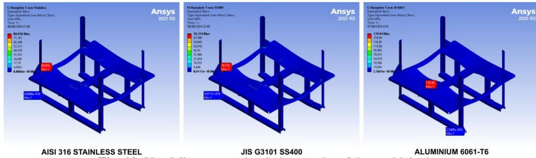
**Fig. 10.** Von Mises stress simulation results of 5 mm-thick plate
