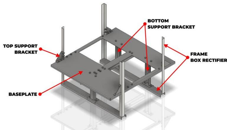
Fig. 2. 3D Design of baseplate
