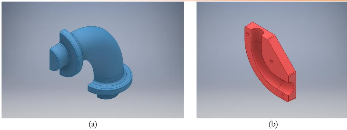
Fig. 3. Pattern design of (a) Intake manifold; (b) Core box
