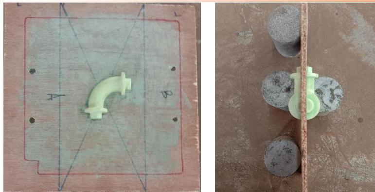
**Fig. 3.** Assembled patterns in wood plate
