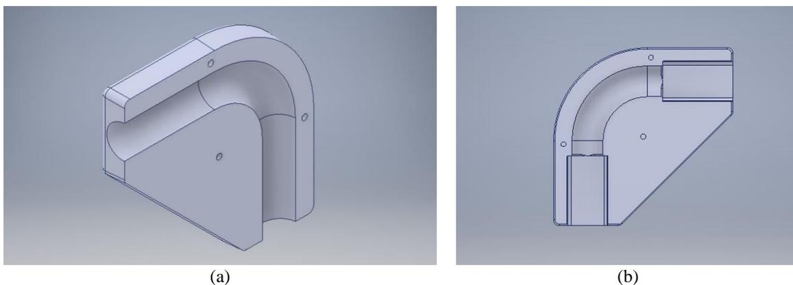
**Fig. 7.** Revision of core box patterns on (a) Cope; and (b) Drag.
