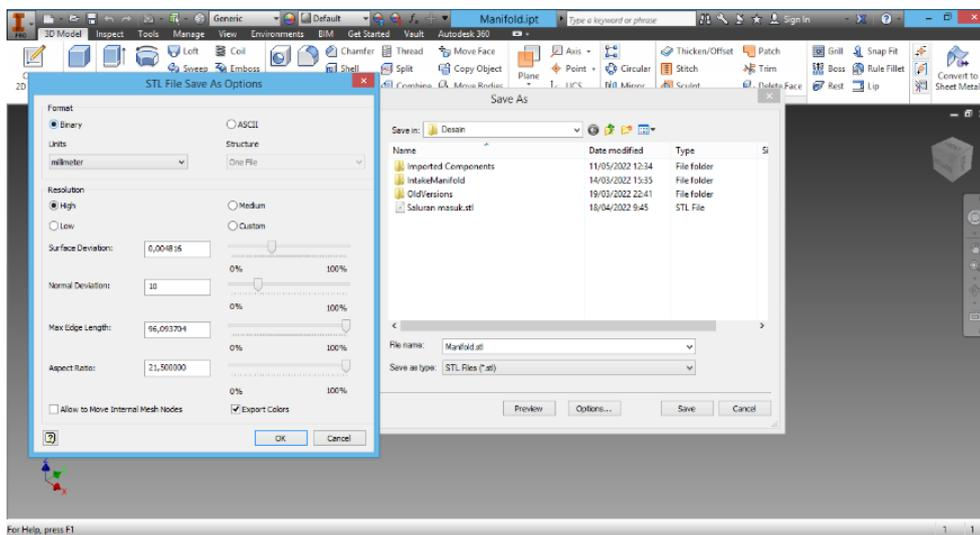
Fig. 4. Converting from IPT format to STL format
