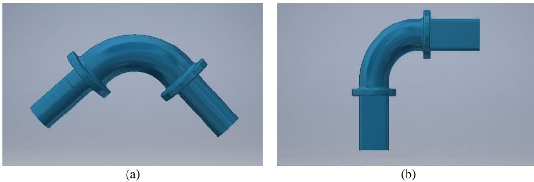
**Fig. 6.** Revision of patterns on (a) Cope; and (b) Drag.
