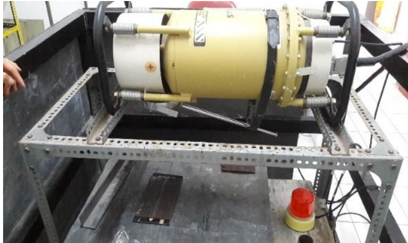
Fig. 2. Radiographic test equipment on welding specimens.
