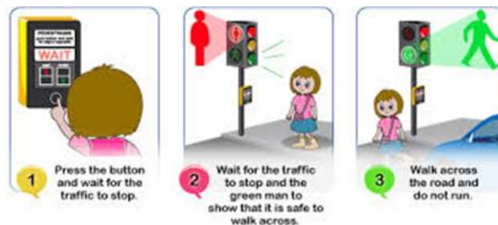
Gambar 16. Cara Kerja Pelican Crossing [1]
